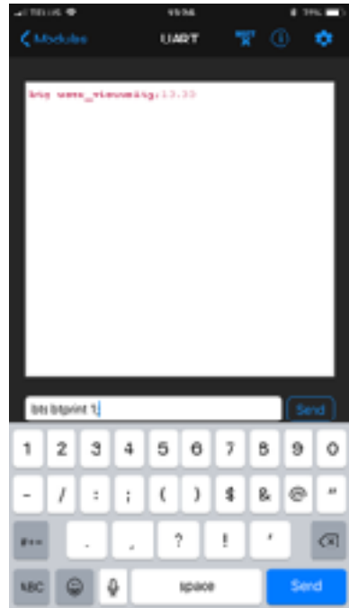
Entering the command "bts BTPRINT 1;" creates a continuous ASCII dump to the screen.
