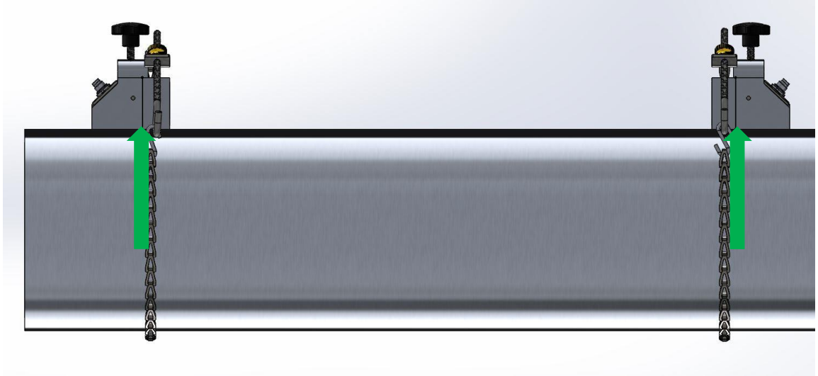
Figure 2-5. Spacing Locating Points on Large Clamps
