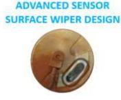
Sensor shown with oil film adhering to sensor, but optics are kept clean with automatic wiper function
