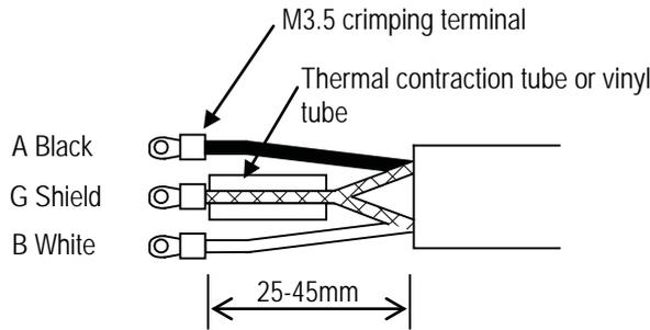
**Figure 5.8 Terminal Treatment of Flow Rate Signal Cable**
