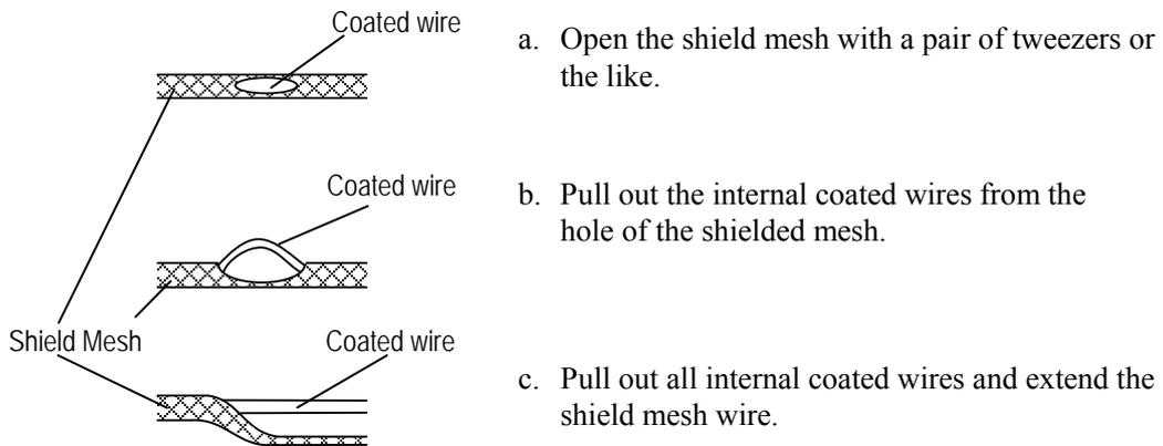
**Figure 5.9 Treating the Signal Cable Shield Mesh**
