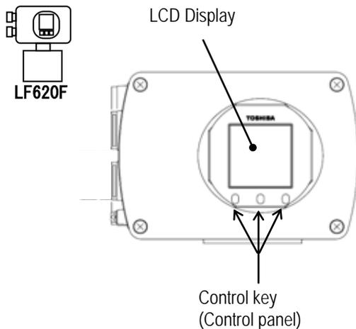
Fig. 7.1 Display section of LF620F
