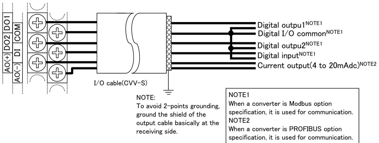
Figure 5.2.1.2 Input and Output Cables Wiring of the LF620F Integral Type Converter
