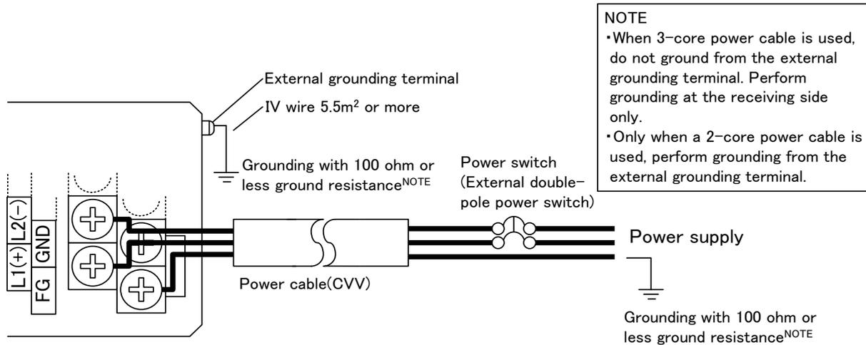
Figure 5.2.1.1 Power Cable Wiring of the LF620F Integral Type Converter
