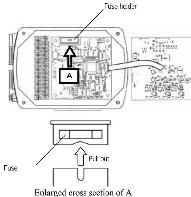
Please use a multimeter to test the conductivity of the fuse.
