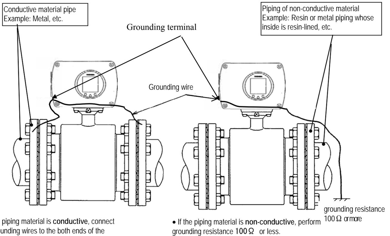
**Figure 5.3 Grounding the LF620F Type**
