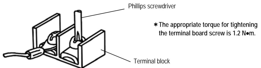
**Figure 5.10 Connecting a Cable to Terminal Block**
