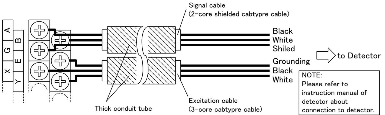
Figure 5.2.2 External Wiring of the LF622F Separate Type Converter
