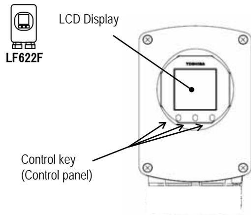
Fig. 7.1 Display section of LF622F
