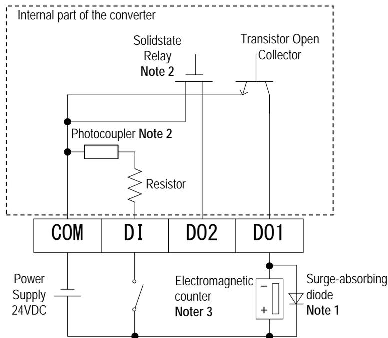
**Figure 5.11 Electromagnetic Counter Connection Example**
