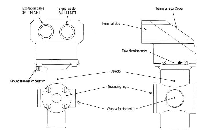
**Figure 3.1.9 Appearance of LF414** Meter size 1/2inch(15mm)
