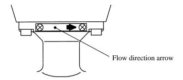
Figure 4.7 Flow direction arrow on the detector
