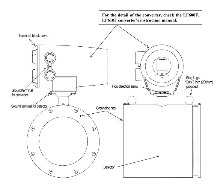
Figure 3.1.4 Appearance of LF414/LF600F, LF610F Meter size 6 and 8 inch(150 and 200mm)
