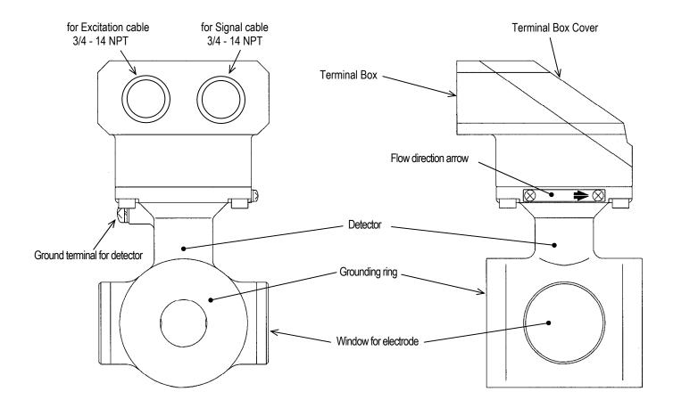
Figure 3.1.10 Appearance of LF414 Meter size 1 inch(25mm)
