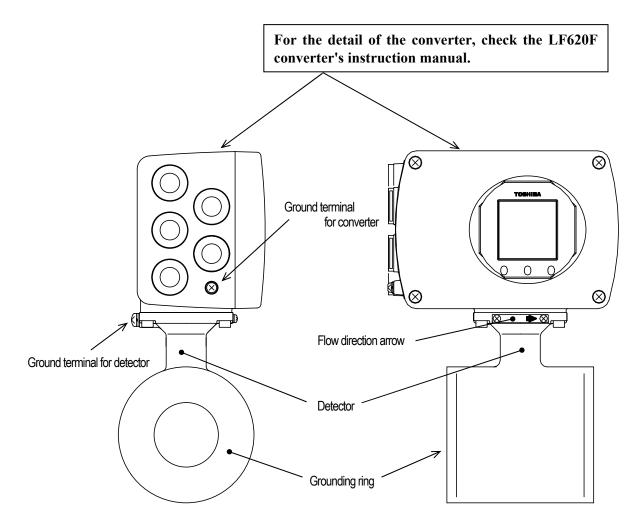
Figure 3.1.7 Appearance of LF414/LF620F Meter size 1 1/2 to 4 inch (40 to 100mm)
