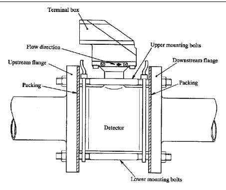
Figure 4.4 LF414 flowmeter detector piping connections
