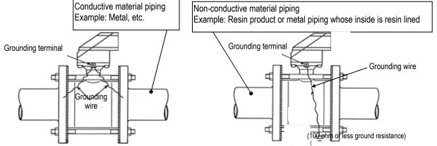
• If the piping material is conductive, connect the grounding wires to the both ends of the piping flange.
