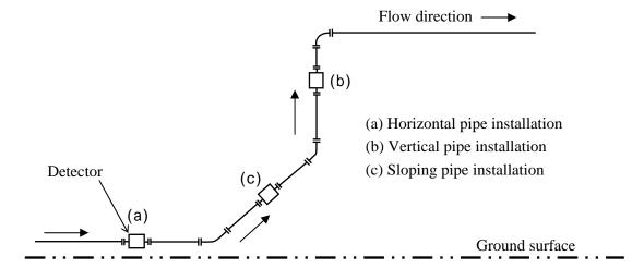
**Figure 4.5 Detector Piping Orientation**
