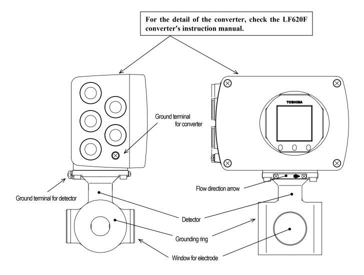
Figure 3.1.6 Appearance of LF414/LF620F Meter size 1 inch(25mm)
