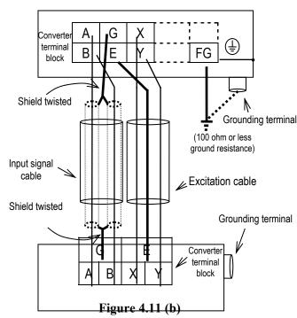
Wiring between Detector and Converter (when grounidng of the detector is difficut)
