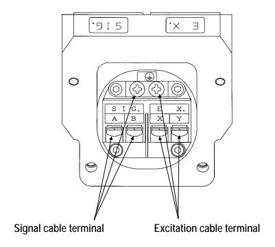
Figure 3.2 Terminal Block of LF414
