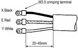
Figure 5.2 Terminal Treatment of Excitation Cable
