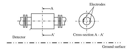
Figure 4.6 Installation position of the detector
