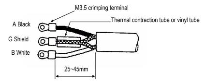
Figure 5.3 Terminal Treatment of Flow Rate Signal Cable
