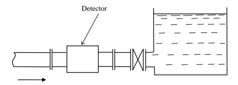
Figure 4.9 Detector with sufficient head pressure at downstream outlet
