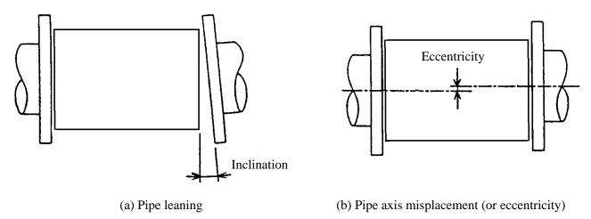
Figure 4.1 Pipe leaning and axis misplacement
