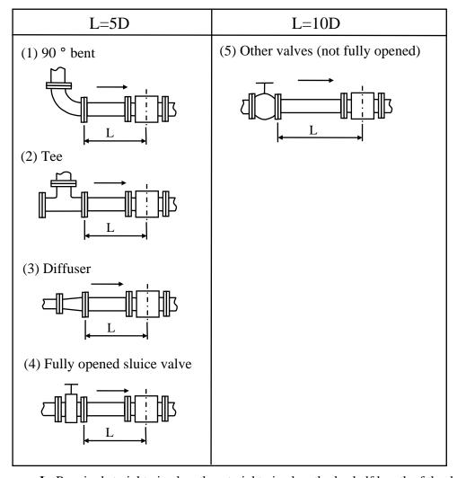
L: Required straight pipe length—straight pipe length plus half length of the detector.
