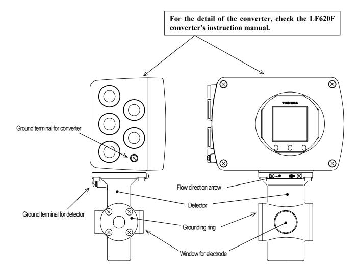
**Figure 3.1.5** Appearance of LF414/LF620F Meter size 1/2inch(15mm)
