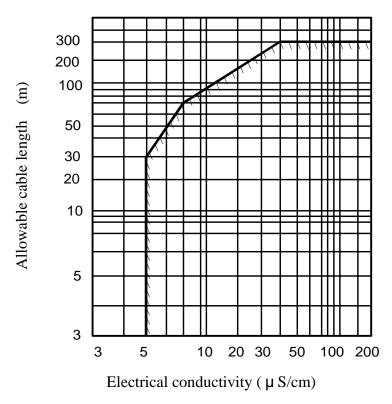
Figure 9.1 Electrical Conductivity vs. Cable Length
