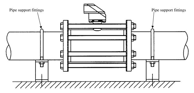
Figure 4.2 Example of Pipe Fixing Procedure
