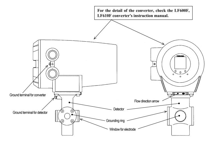
Figure 3.1.1 Appearance of LF414/LF600F, LF610F Meter size 1/2inch(15mm)
