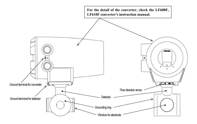
Figure 3.1.2 Appearance of LF414/LF600F, LF610F Meter size 1 inch(25mm)
