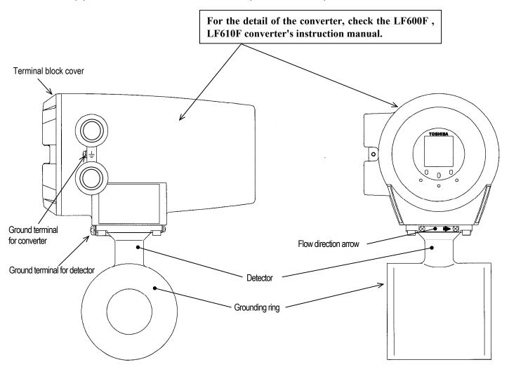
Figure 3.1.3 Appearance of LF414/LF600F, LF610F Meter size 1 1/2 to 4 inch (40 to 100mm)
