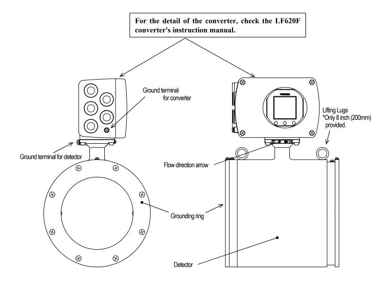
Figure 3.1.8 Appearance of LF414/LF620F Meter size 6 and 8 inch (150 and 200mm)
