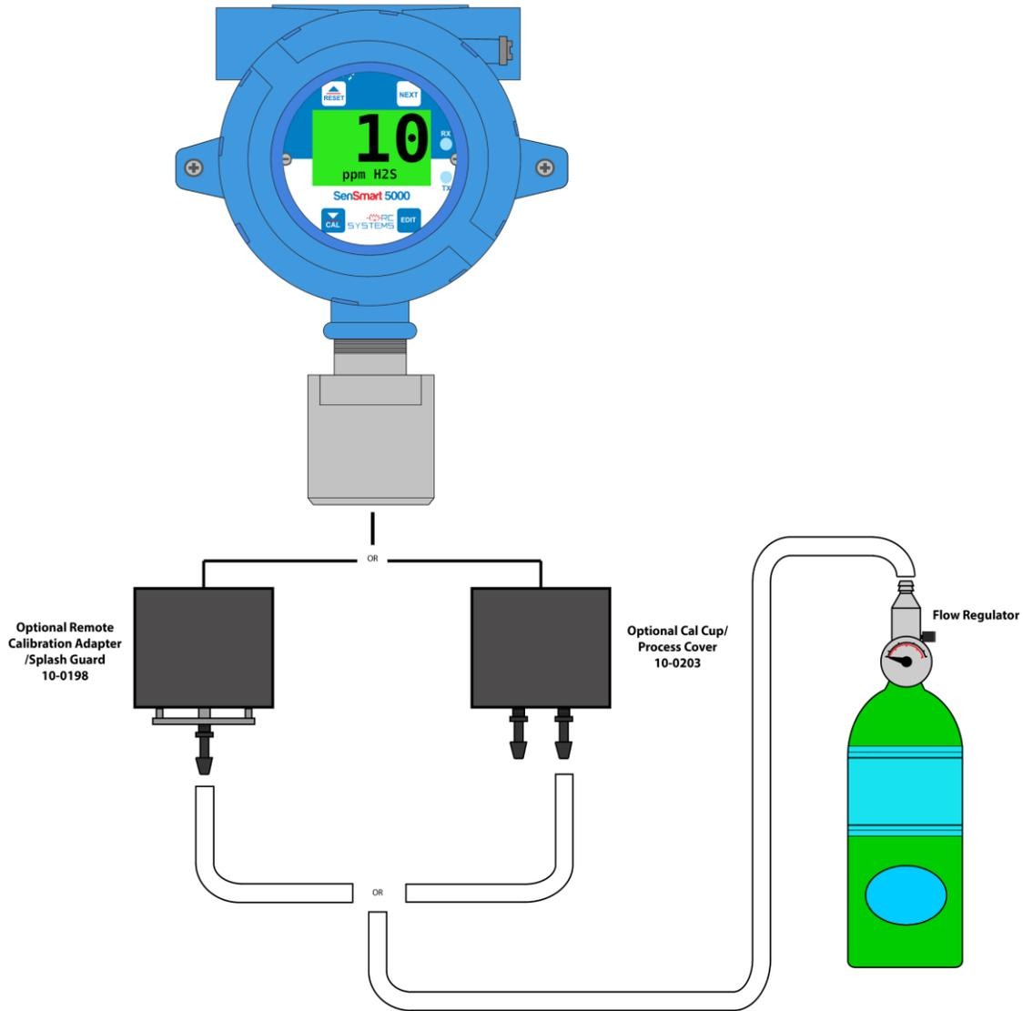
Figure 12 Calibration Diagram
