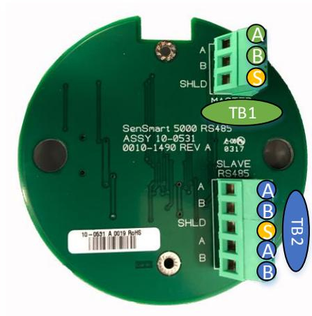
*Figure 4 SenSmart 5000 Modbus Option Wiring*
