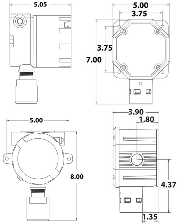
Figure 15 Mounting Dimensions
