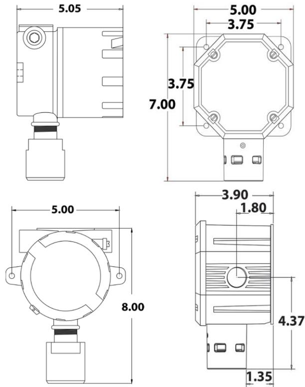
*Figure 1 Mounting Dimensions*
