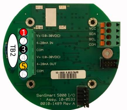
Figure 3 SenSmart 5000 Wiring
