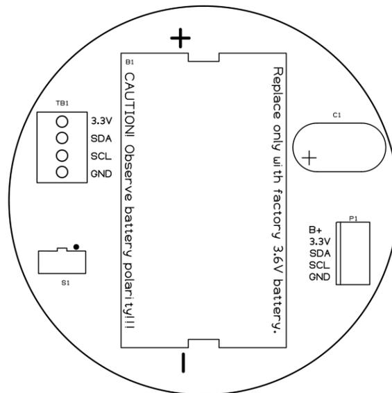
Figure 23 10-0534 Battery Board
