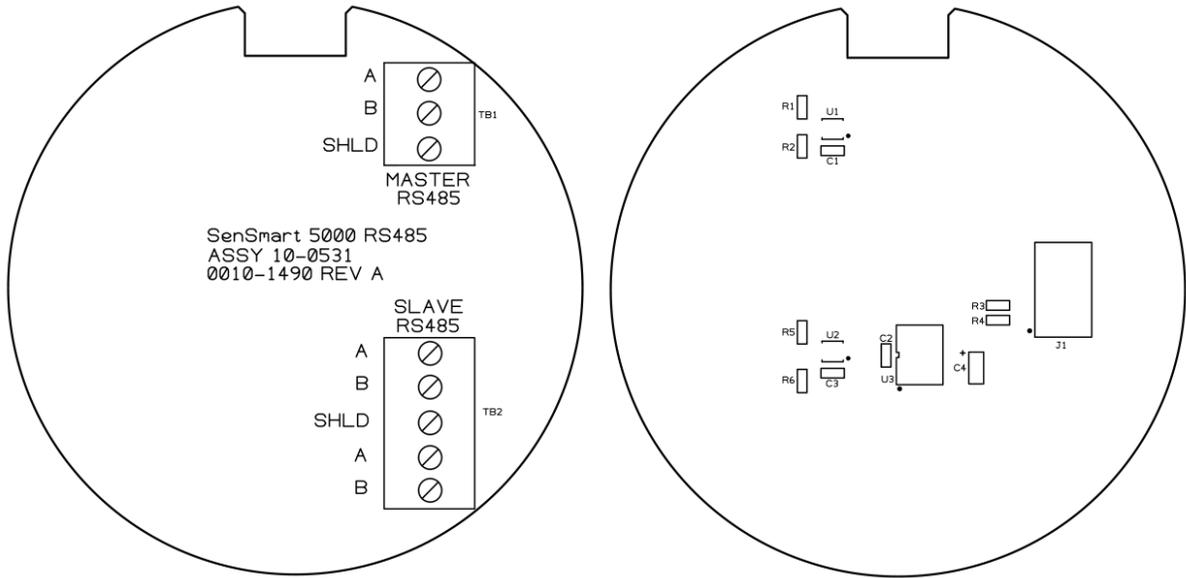
Figure 18 10-0531 Modbus Board
