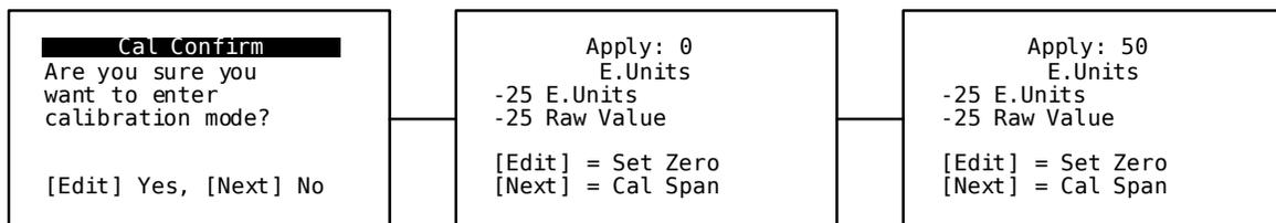
Figure 13 Calibration Menu Flowchart
