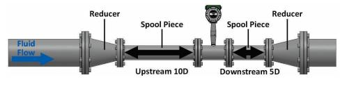
M24R Reduced Bore Vortex with integrated reducing flanges
