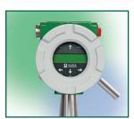
VorTek Instruments Pro-V™ M24 Multivariable Vortex Flowmeter offers accurate and reliable flow metering in a multivariable design. The multivariable design incorporates a high-accuracy velocity sensor, a precision platinum RTD temperature sensor, and a solid-state pressure transducer. The M24 can deliver volumetric flow, mass flow, temperature, pressure, density, and energy (BTU) measurements
