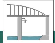
**River level measurement:** To measure levels of rivers used for drinking water or to detect flooding conditions caused by dam releases or inclement weather.
