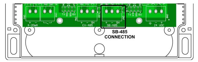
The SB-485 connection (CN7) is a three wire terminal block located near the center of the printed circuit board and is for connection to the SmartBob RS-485 network. Two terminal screws marked + and – should be connected to the positive and negative wires of the SmartBob network cable. The third terminal screw marked SH should be connected to the shield of the SmartBob network cable. Do NOT connect the shield to earth.
