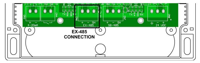
The EX-485 connection (CN6) is a three wire terminal block located near the center of the printed circuit board and is for connection to the Expansion RS-485 network. Two terminal screws marked + and - should be connected to the positive and negative wires of the RS-485 network cable. The third terminal
