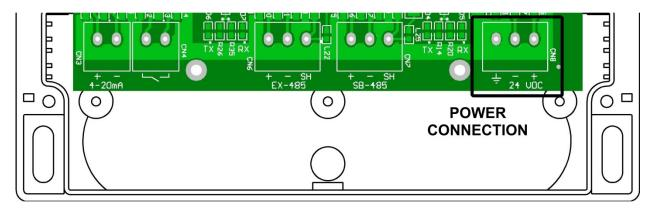
The power connection (CN8) is a three wire terminal block located on the far right. Two terminal screws marked + and - are for connecting to a 24VDC source, isolated from earth ground. See section 2.0 Specifications for power source requirements. Due to the low power requirements of this console, a 16 or 18 AWG wire would be sufficient for these two power connections.
