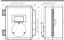
Note: Drawings above are shown with the optional splash quard. Without the splash guard, the thickness of the unit is 71 mm (2.8 inches).
