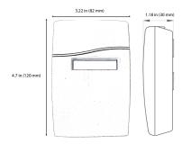
AST-IS14 (measurements are in mm and inches)
