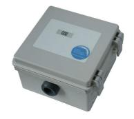
The AST-I series of analog transmitters are high quality, industrial, dual beam, referenced transmitters with miniature infrared sensors, analog output and water / dust tight, corrosion resistant, non-metallic enclosures.
