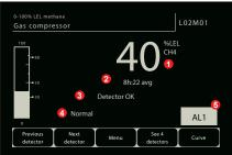
Current value with unit and detected gas
