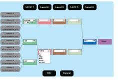
1 Simple relay programming 2 Up to five embedded functions: OR, AND, NOR, NAND, VOTING
