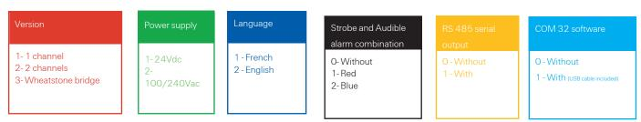
f.i: MX32-1-2-2-1-1 for MX32 1 channel, 100/240Vac, English, Blue strobe & horn, RS485 output and COM 32 software
