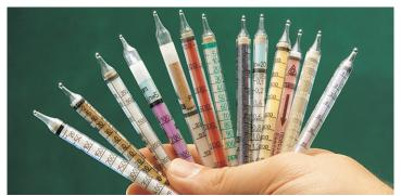
KWIK-DRAW<sup>™</sup> detector tubes are a reliable method of spot testing for more than 200 hazardous gases and vapors. The highly sensitive detector tubes are designed for evaluation of the potential presence of ultra toxic chemical substances in the air and are resistant to interfering substances.
