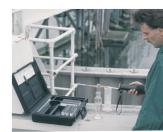
The water analysis kit permits a quick and easy determination of volatile substances such as perchloroethylene, benzene, etc., in a water sample. A detector tube pump is necessary for the use of detector tubes (KWIK-DRAW™ Gas-Tester, Gas-Tester II H, Toximeter II)
