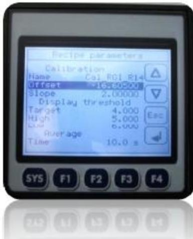
Access to this screen is locked by the user password. This password is changed by the administrator in the Administrator screen. Only useful process parameters can be changed on this screen. For other parameters, using the PC XIR NIR. To change a setting, move the selection on the corresponding line and press the "Enter" key. Enter the new value and exit the screen with the "ESC" key. See the manual for use XIR parameters.
