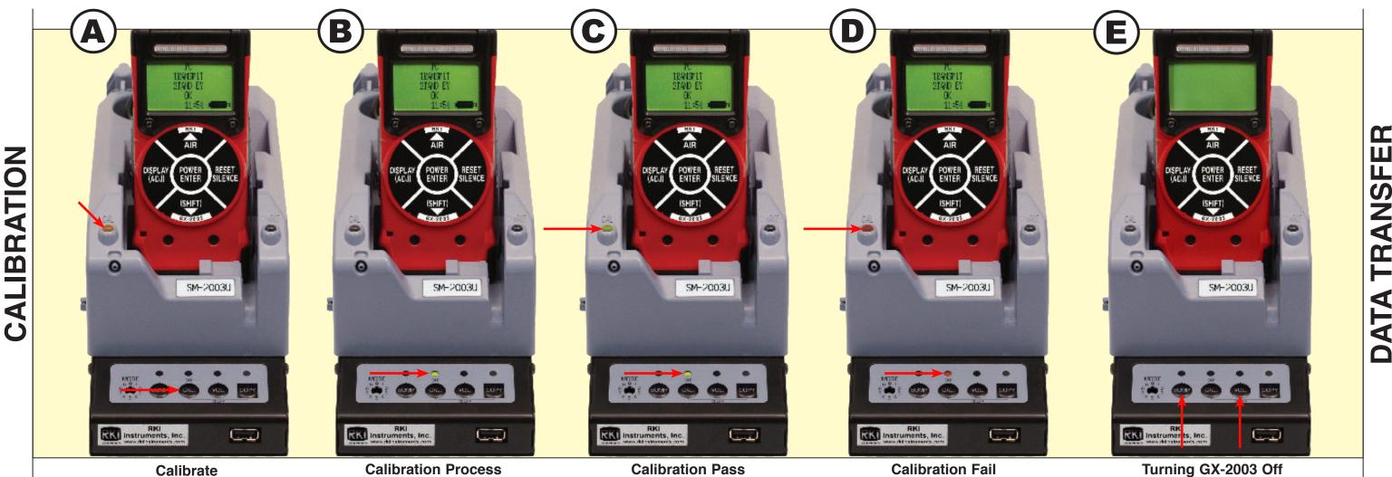
Power Instrument on. After CAL LED light is steady orange, press the "CAL" button to start calibration.
