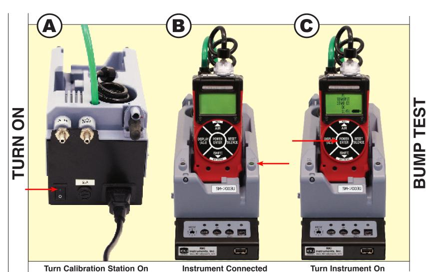
Attach power cord to back of cal station. Press the power button at the back of the cal station to the
