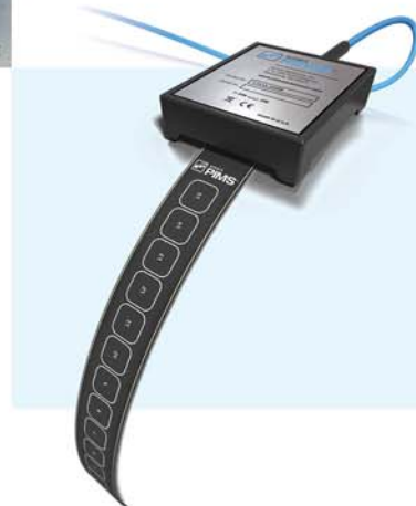
Flexible matPIMS linear or area arrays, with 16 ultrasonic elements can be wrapped around pipes and elbow extrados, with up to 1,000' (305 m) of cable.
