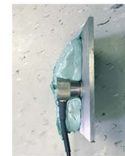
For long-term installations, including underground or harsh environments, the transducer is encapsulated for extended protection.
