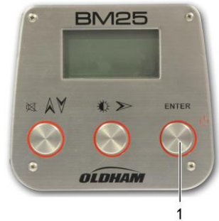
Figure 19: switch off by pressing Enter button
