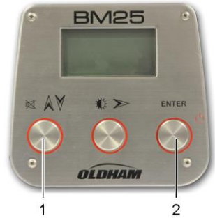
Figure 14: press 1 and 2 to select the calibration gas
