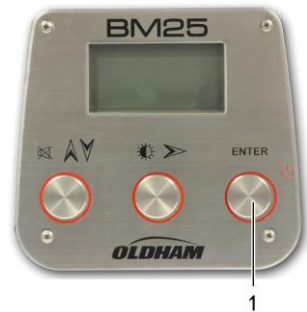
Figure 13: start-up in standard mode by pressing the Enter button
