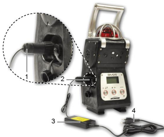
Figure 10: charging in safe area
