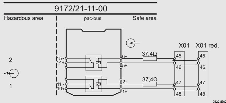
The selected version of the loop-powered binary output is based on the field device to be connected.
