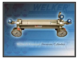
The Constant Pressure Sample Cylinder is designed for use in systems where it is necessary to extract and isolate accurate product samples by maintaining a steady pressure from the pipeline to the cylinder. The cylinders are equipped with a magnetic indicator and a graduated scale set to specify the capacity of the device.
