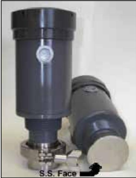
The sanitary models are designed specifically for applications where sanitary standards apply such as in water treatment plants, food and beverage manufacturing, or pharmaceutical processing. These sensors are appropriate for measuring ranges from five inches to 30 feet by using different operating frequencies. The 300 series features a stainless steel mounting adapter and transducer face that is self cleaning to automatically remove any buildup for ease of maintenance.
