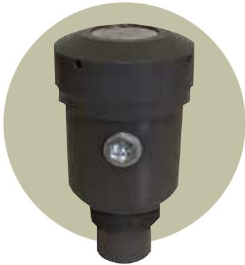
*If only a simple 4 – 20 mA output is required, a two-wire SmartSonic ultrasonic sensor may be utilized. Available in both standard and sanitary models, the two-wire model offers all of the design benefits of SmartSonic technology, but with more limited communications options. Programming is done on the sensor versus via PC software.*
