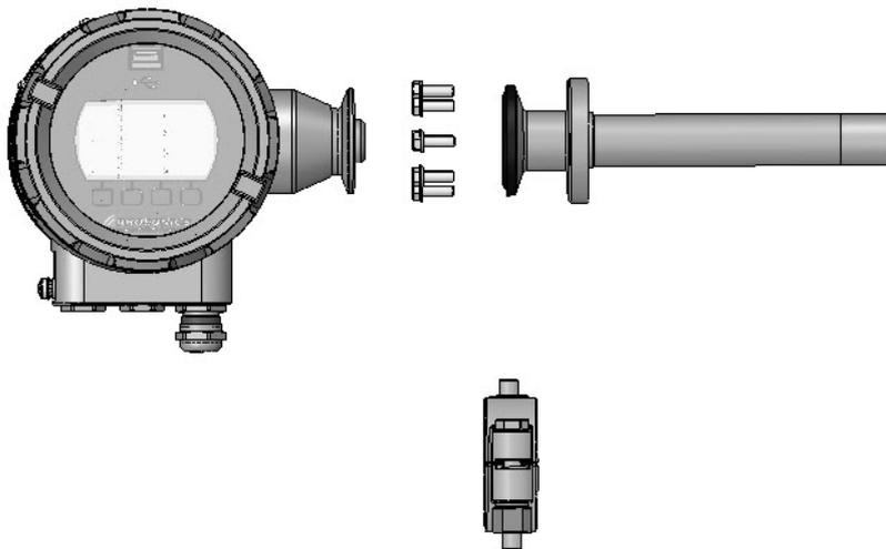
Dismounting: Remove the M5x16 bolts and M5 washers / **Mounting: Place the M5x16 bolts and M5 washers**
