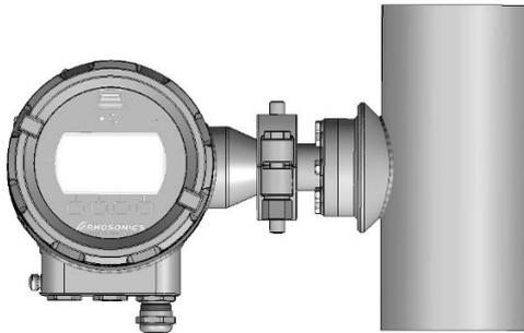
SDM WT mounted in a Weldolet (vertical mount)
