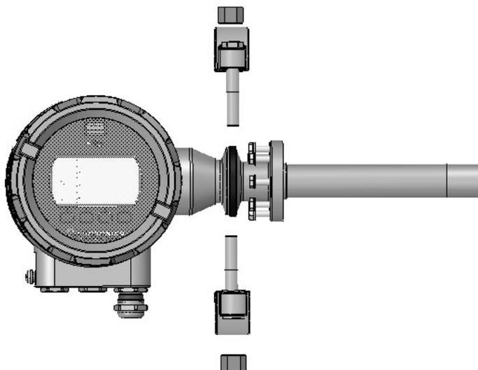
Dismounting: Remove Tri-clamp / Mounting: Place Tri-clamp
