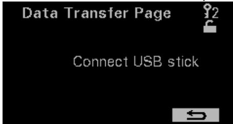
The USB stick is checked. This is followed by saving the echoes and settings and measured values. Within 20 seconds this should be finished. If failed, the display shows so.
