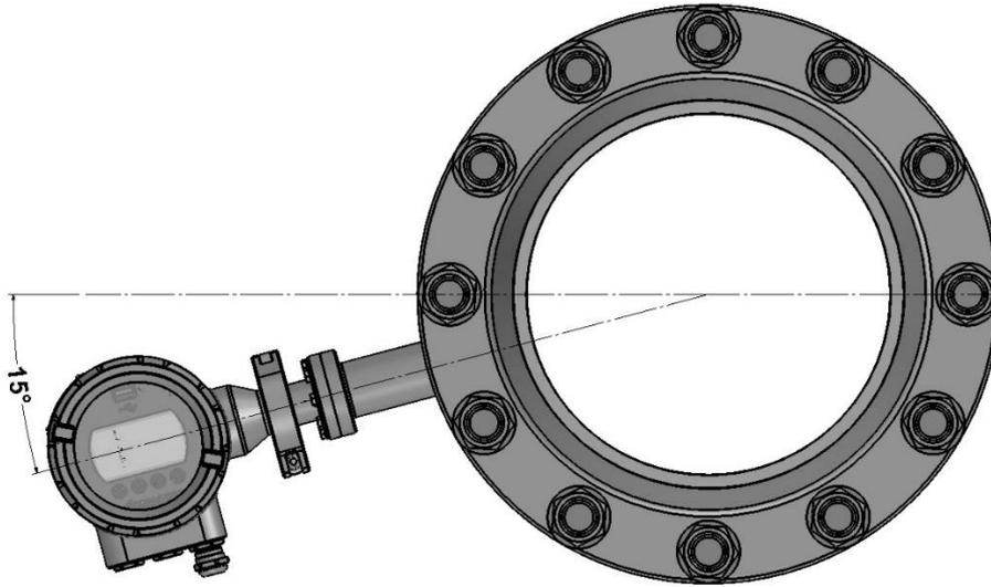
105° Horizontal pipe mounting (i.e. wafer)
