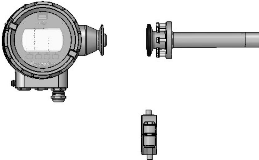
Dismounting: Separate sensor and housing, NOTE take care of the tiny spring loaded contacts in the sensor part / **Mounting: Connect sensor and housing, NOTE take care of the tiny spring loaded contacts in the sensor part**
