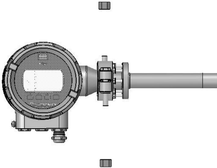
Dismounting: Remove nuts from Tri-clamp / Mounting: Tighten nuts to Tri-clamp with 25 Nm
