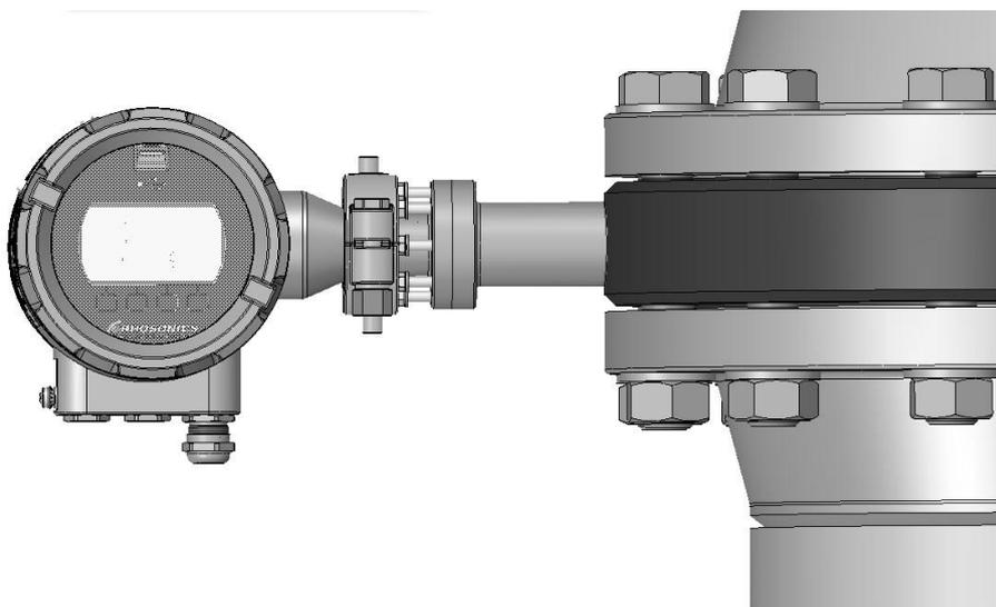
Dismounting: Untighten 8 M5x16 bolts / Mounting: tighten bolts with 4.2 Nm
