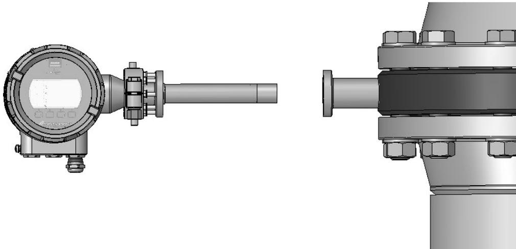
Dismounting: Remove sensor from pipe(adapter) / Mounting: place sensor into pipe(adapter)
