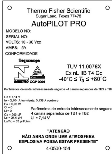
Figure 3–15. Flow computer certification tag for hazardous area (Brazil)
