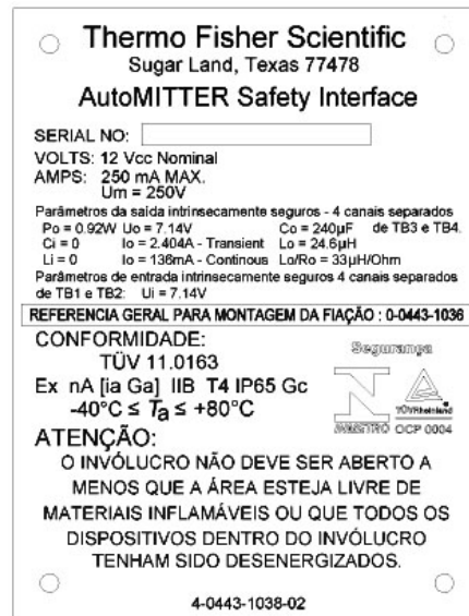
Figure 6–6. Certificate marking for Brazilian installations
