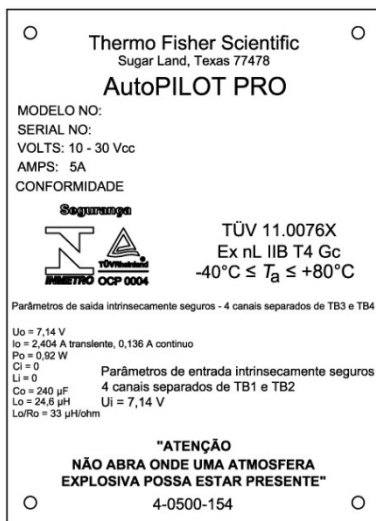
Figure 3–15. Flow computer certification tag for hazardous area (Brazil)
