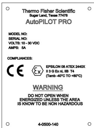
Figure 3–14. Flow computer certification tag without AutoMITTER SIB option
