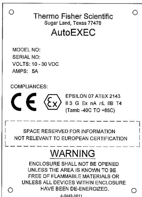
Figure 3-11. Flow computer certification tag for hazardous area
