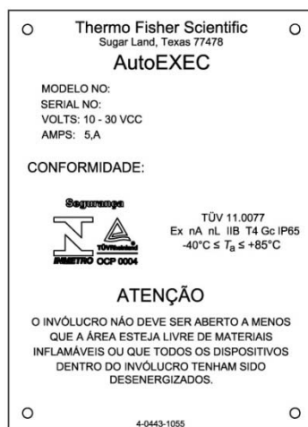
Figure 3–12. Flow computer certification tag for hazardous area (Brazil)
