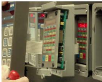
2. Remove S3+ front assembly
