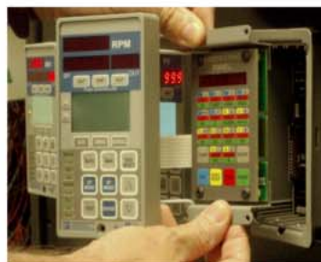
5. Replace with S3++ front assembly
