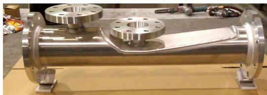
Experimental meter for density and tap design laboratory studies
