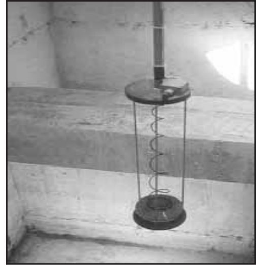
ID-223/500 installed in a flow stilling outlet tank, monitoring oil/water separator discharge.
